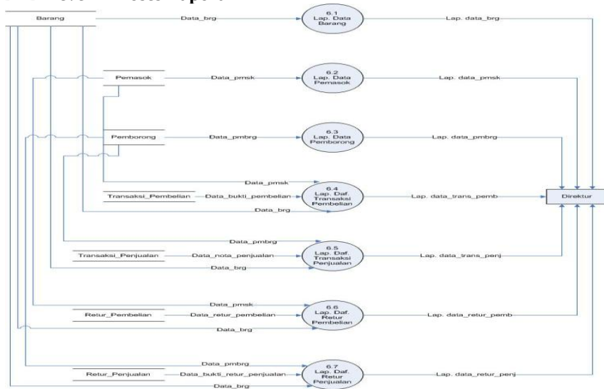
Gambar 8. DFD Level 1 Proses Laporan
