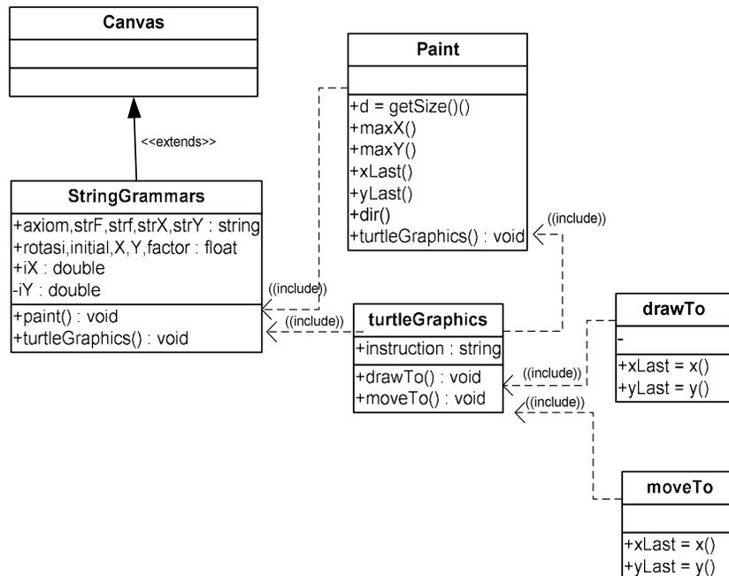
Gambar 17. Class diagram String Grammars
