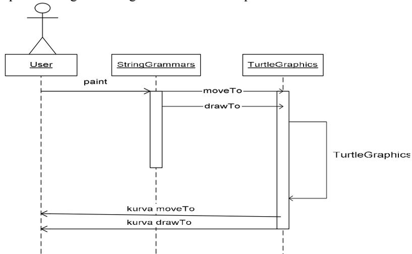
Gambar 18. Sequential diagram String Grammars
